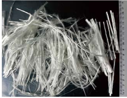
Recycled fibers recovered using Gjenkraft's thermal recycling process
