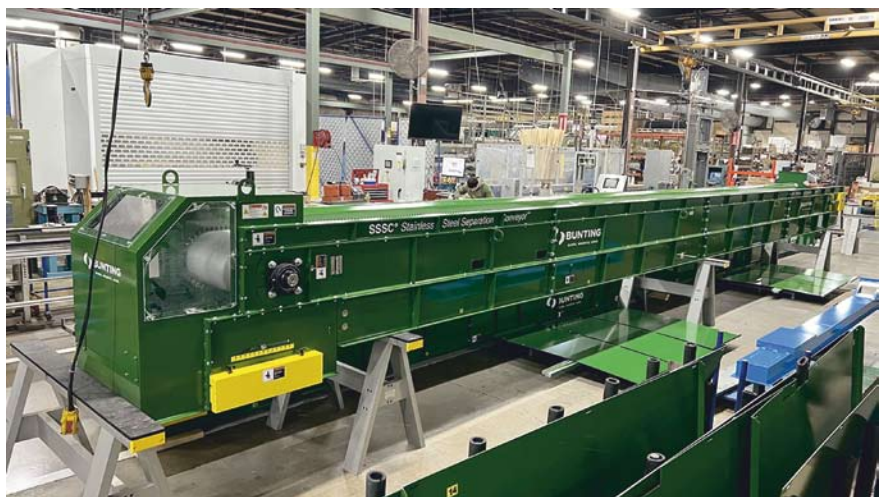
The 11.6-metre long SSSC 12-24-462 Stainless Steel Separation Conveyor
